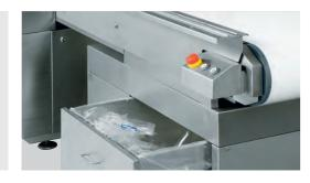
Complete cut-off means that the protruding bag material of the packages is cut off directly in the vacuum chamber. The exhaust system sucks the bag remains into an external container located underneath the loading belt so manual removal of the excessive bag material is no longer necessary.
