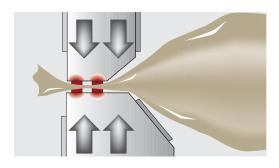
The double biactive high-pressure sealing and the spring-loaded resistance wires are standard equipment and ensure safe and reliable seals despite folds, fats, oils or moisture in the seal area. Springs keep the resistance wires in the correct track even with continuous operation.
