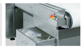
Complete cut-off means that the protruding bag material of the packages is cut off directly in the vacuum chamber. The exhaust system sucks the bag remains into an external container located underneath the loading belt so manual removal of the excessive bag material is no longer necessary.
