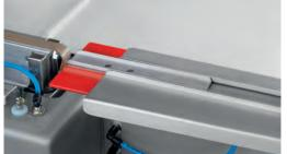
**Water-cooled sealing bars** increase the durability of the Teflon and the sealing wires.
