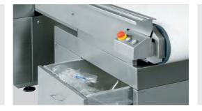
**Complete cut-off** means that the protruding bag material of the packages is cut off directly in the vacuum chamber. The exhaust system sucks the bag remains into an external container located underneath the loading belt so manual removal of the excessive bag material is no longer necessary.
