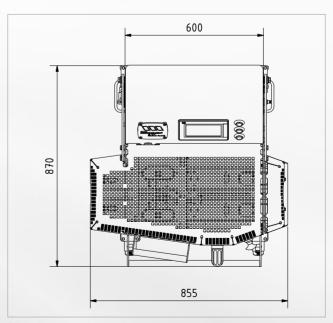
The beginning of the sausage chain is - either automatically or manually – inserted into the link cutter type WKT-50 and the system automatically feeds the other sausages gradually. The machine is able to precisely recognize the twist point even with different sausage types. Various product and machine parameters can be set in advance. Very long sausages can - if requested by the customer - also be cut into pieces.
