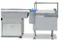
**Corner transfer unit** including control box and sensors designed for loading the belt machine on one or both sides.
