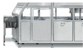
**Rotary table** including housing. Every second product is rotated 180° and can thus be optimally prepared for loading into the belt machine so that the bag ends are always facing outward.
