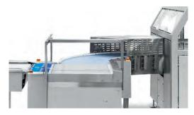
**Curved conveyor belt** including housing. Connection between rotary table and corner transfer unit.
